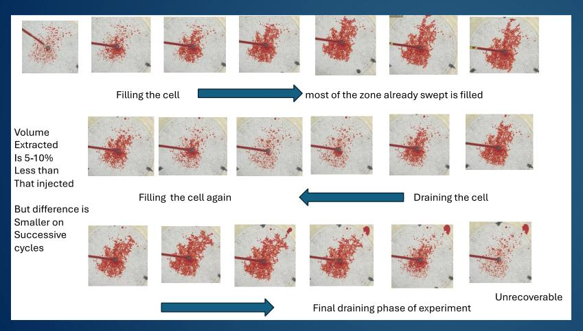
Initial experiments involve flowing coloured water into oil saturated bead pack
