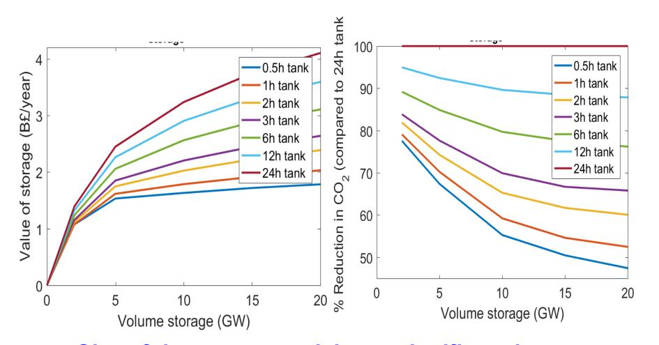
Size of the storage tank has a significant impact for large volumes of deployed storage capacity
