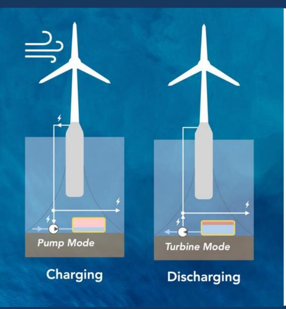
Combining pressurised seawater and compressed air
