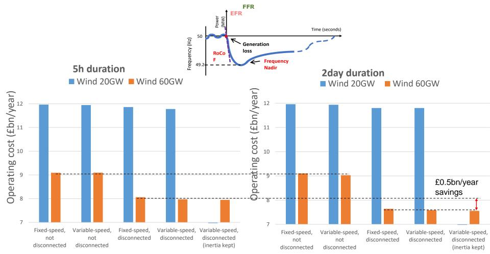
Assuming that ES units in charging mode could **provide fast frequency response** by disconnecting after an outage, and potentially **provide inertia**
