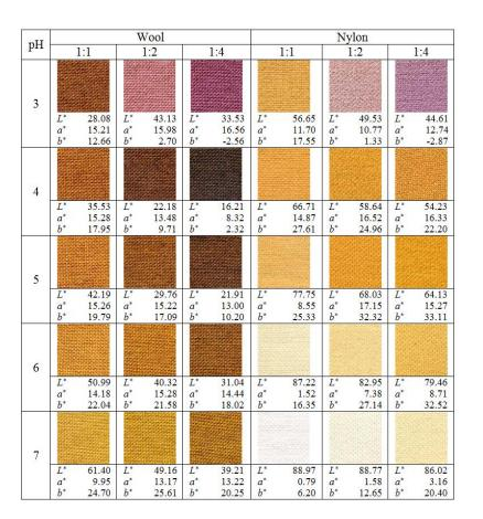
Wool and nylon fabrics dyed in-situ by laccase with a 2,5 DABS precursor under different pH
