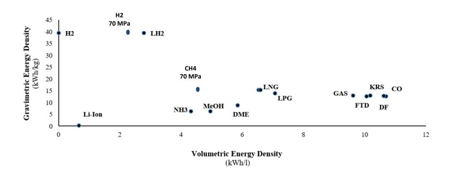
Where: GAS is gasoline, KRS is kerosene, DF is diesel fuel and CO is crude oil.
