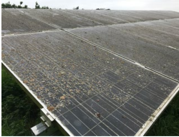
Soiling of module cover glass in a UK solar utility (image courtesy of Solar Farm Cleaning)
